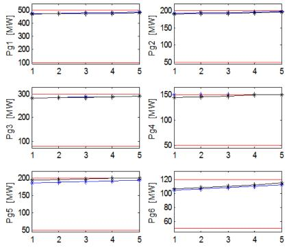
Fig.6. Generation power at each generation bus, (blue) using lagrange method and (black) using the proposed method.
