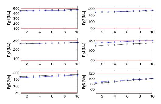
Fig.2. Generation power at each generation bus, (blue) using lagrange method and (black) using the proposed method.
