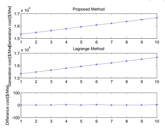
Fig.1. Total generation cost using Lagrange method and the proposed method and the difference between them.
